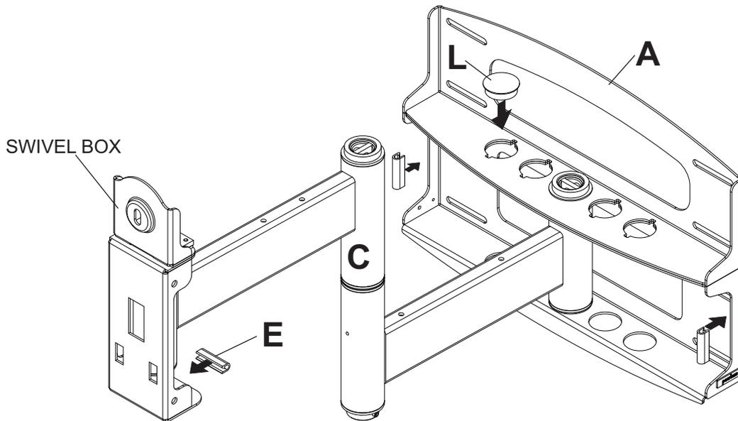
**Note:** Refer to adapter bracket instruction sheet for attachment of adapter bracket to plasma before proceeding with step 5. If your adapter bracket has an aluminum race attached to it, remove before proceeding and discard race. It is not used with this product.
